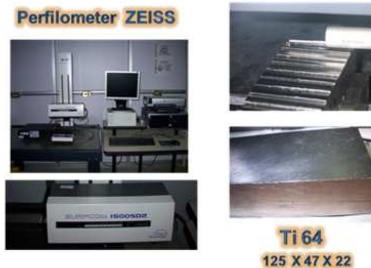
Figure 5. Profilometer Surfcom 1500SD2.
