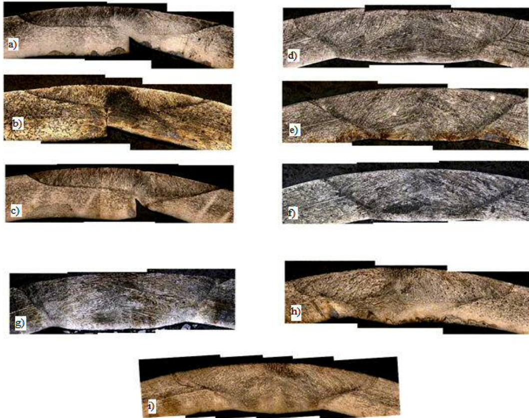
**Figure 4.** Metallographic profile of welded samples **a)** travel speed 335.28m/h, 0% $H_2$  **b)** travel speed 350.52m/h, 0% $H_2$  **c)** travel speed 365.76m/h, 0% $H_2$  **d)** travel speed 335.28m/h, 6% $H_2$  **e)** travel speed 350.52m/h, 6% $H_2$  **f)** travel speed 365.76m/h, 6% $H_2$  **g)** travel speed 335.28m/h, 12% $H_2$  **h)** travel speed 350.52m/h, 12% $H_2$  **i)** travel speed 365.76m/h, 12% $H_2$ .
