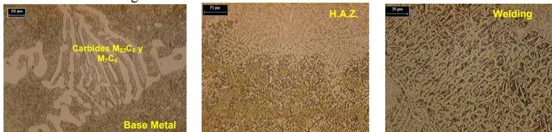
**Figure 3.** Tempered martensite with carbides  $M_{23}C_7$  and Chromium and Molybdenum matrix dispersed  $M_7C_6$ .
